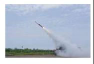
a range of around 25 to 30 km with 2 vehicle configuration for area air defence. It is a truck-mounted missile with a 360 degree rotatable, electro-mechanically operated, turret-based launch unit.
